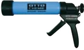
Heavy duty hand-operated gun made of highly impact-resistant plastic, very lightweight. With closer for sliding sleeve, smooth driving rod and sliding sleeve for 290/300/310 ml cartridges. Automatic pressure relief.
