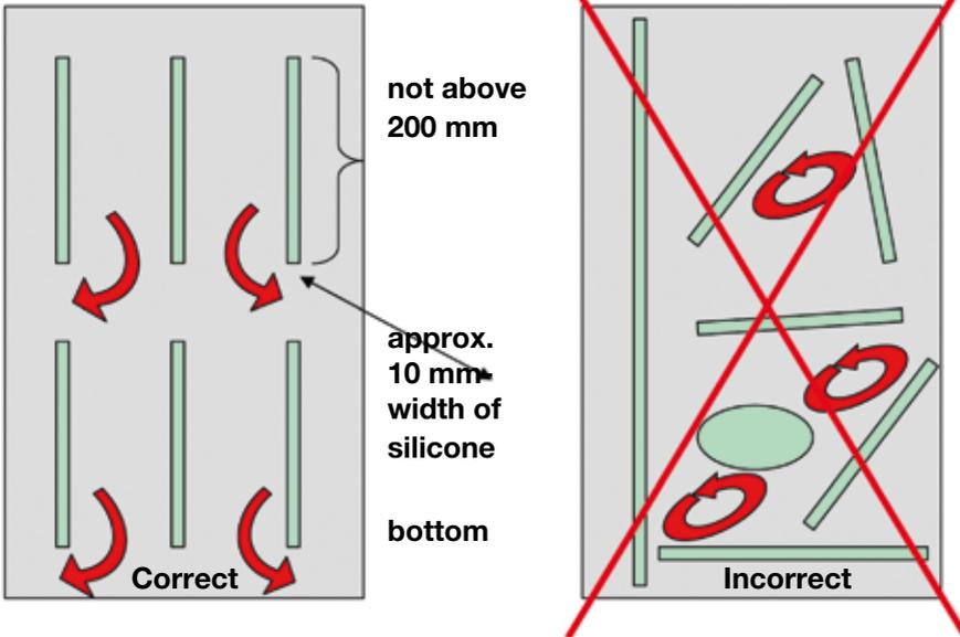
In order to avoid the confinement of the splitting product, a minimum space of 1,6 mm between mirror and substrate has to be kept mandatory. This space can be avoided most purposefully by sticking spacers onto the mirror. It does however not overrule the minimum distances for ventilation given by the Institute of Glass Manufacturing in Hadamar ([www.glashandwerk.de](http://www.glashandwerk.de)).
